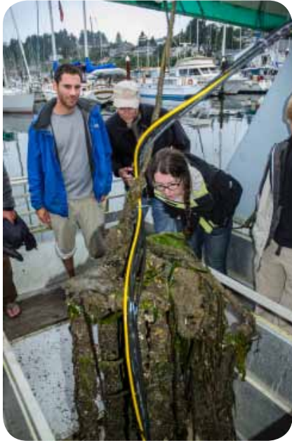
Photo left: Math Camp students Allan Lerner and Allison Einolf (left and right) and Teaching Assistant Steve Drake (middle) looking at the extensive biofouling of the LOBO (Land/Ocean Biogeochemical Observatory) mooring in Yaquina Bay from which long-term time series of salinity, nitrate and turbidity were analyzed as part of the course material in Math Camp.
