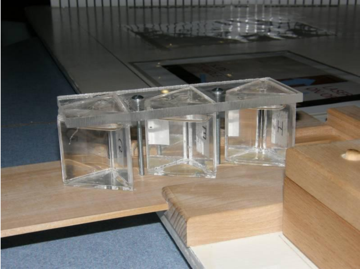
Fig 6 Detail of prisms, top strap and bolts
