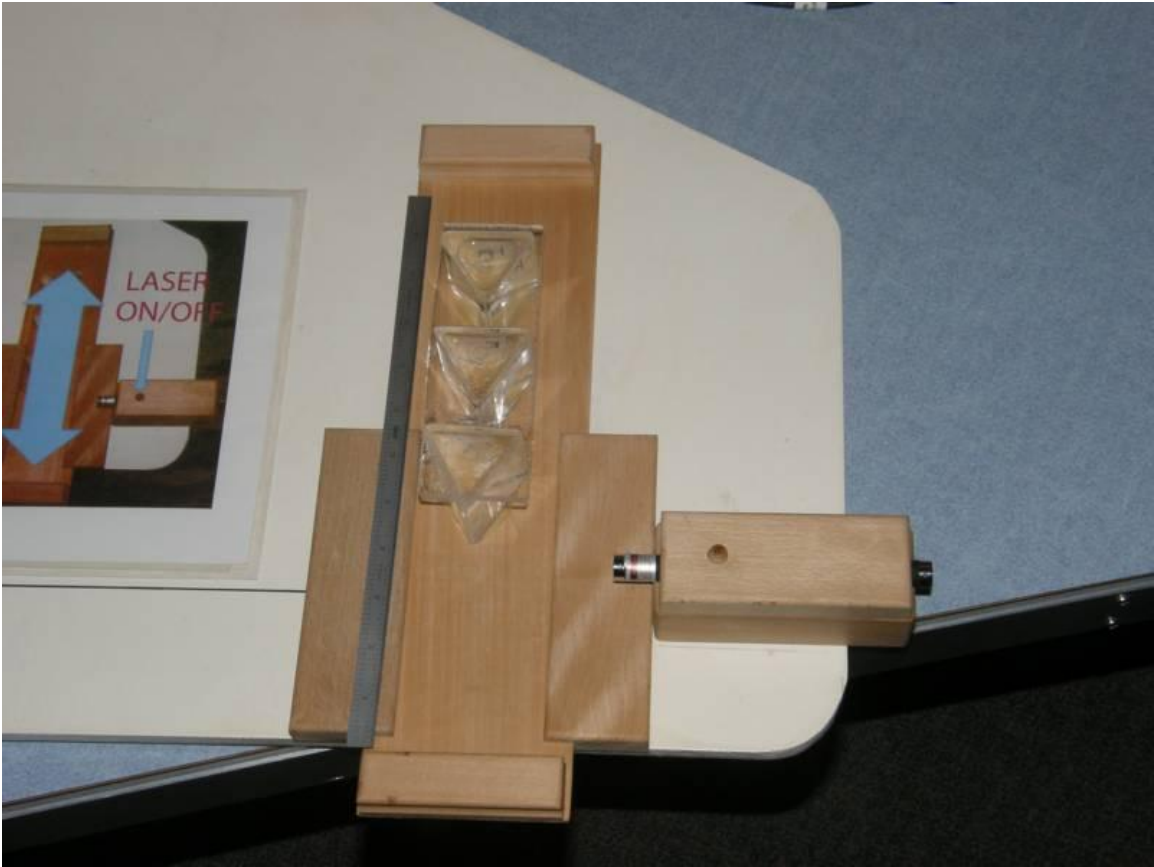
Fig 4 Finished prism slide, slide holders and laser cradle
