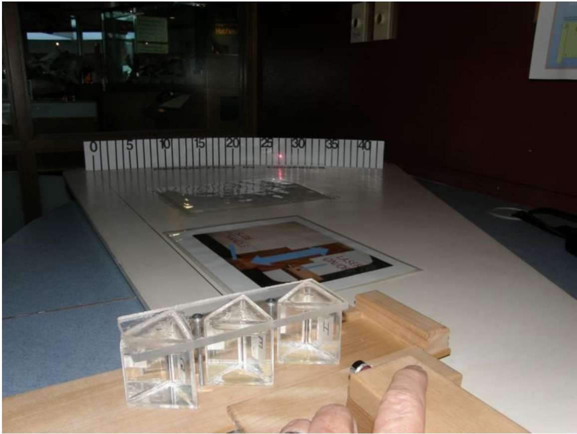
Fig 7 Refractometer in operation The angle shown is about 27.1 degrees
